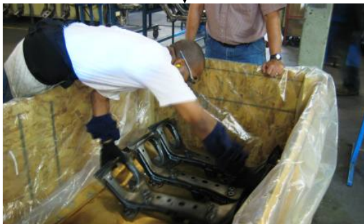
3. Place one layer of cooled parts on PW32. Always wear gloves to avoid contamination.
