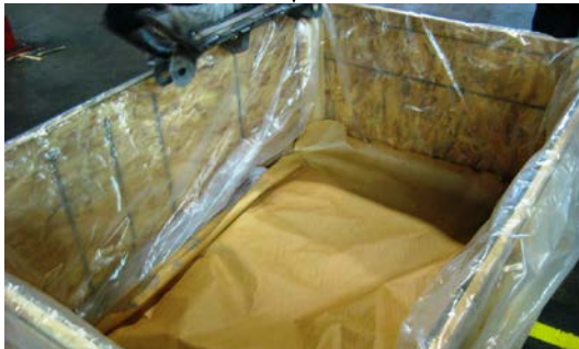
2. Place full size sheet of PW32 at base. Print side down.
