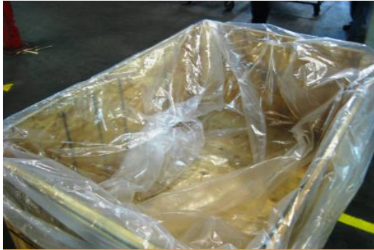
1. Line empty crate with 4 mil polyethylene bag
