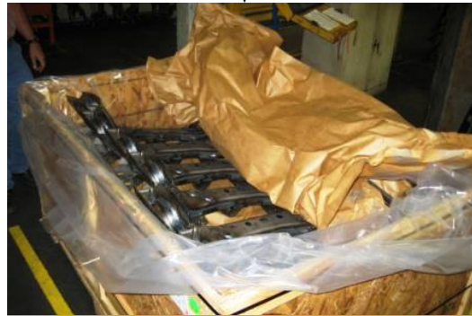
5. Place PW32 over top & bottom of each layer
