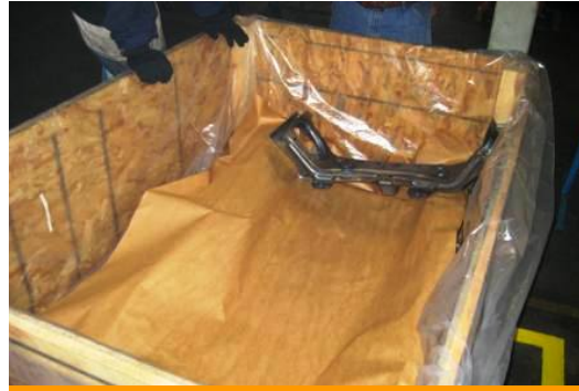
4. Place PW32 over each layer of parts.
